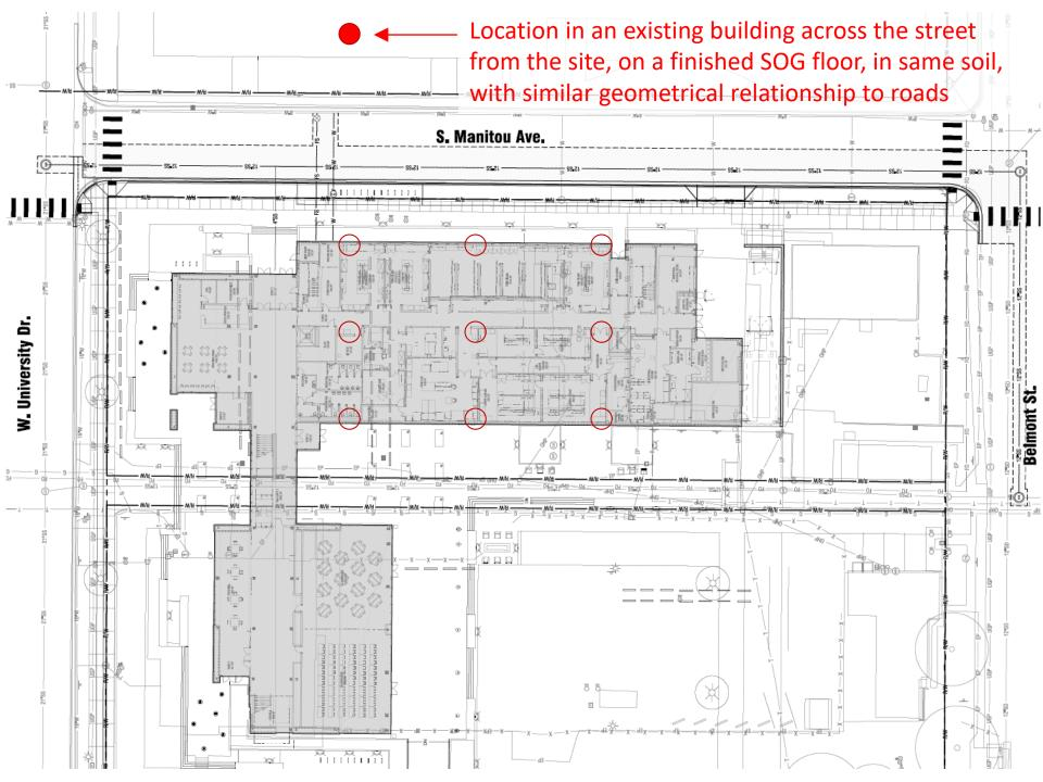
Proposed alternative technique for developing useful ground/building micro-vibration data.
